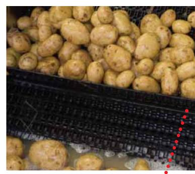
Streamline flights are available up to 6.0 in. (152 mm) and can be cut down to any height required for a particular application.
