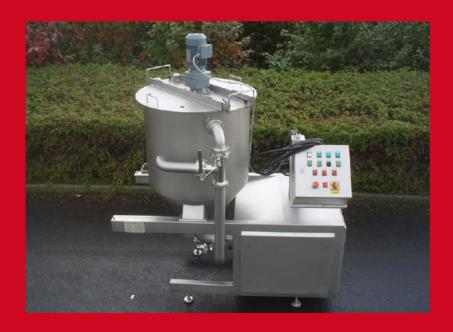
Consequently, mayonnaises of all quality grades, ketchups, spicy sauces, dressings, emulsions, dips, remouladen, soups and other products can be manufactured. For the processing of homogeneous products the machines are supplied without an adjustment unit. The individual ingredients are added either directly into the mixing container or by means of a side funnel.
