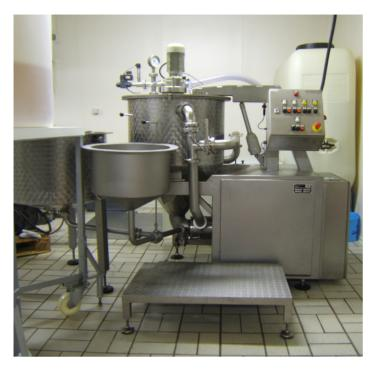
Vacuum mechanisms are available for the series 159 C and 159 G machines. In this case, the homogenising process takes place under vacuum conditions; the product is thereby continuously vented and thus has a longer durability and is protected against oxidation and discoloration.
