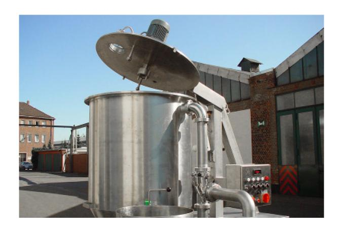
The new 159 M additional unit allows homogenisation and mixing in a single production step by adjusting the perforated discs!
